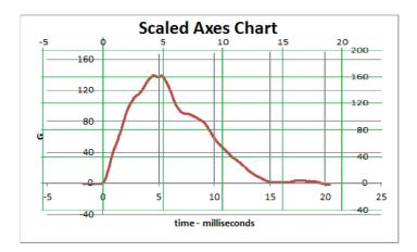
The axes at the bottom and left and the gray grid lines apply to the raw data as collected from the test. The axes at the top and right and the green grid are scaled and apply to the raw data as an approximation of the results which might be obtained if the drop mass and impact velocity had been 5.6 kg and 8.0 m/sec as called out in the standard.
