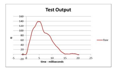
applying the appropriate scale factors to the time and G components of each point will yield:
